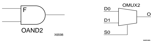
Figure 20: AND & MUX Symbols in XC4000X IOB
