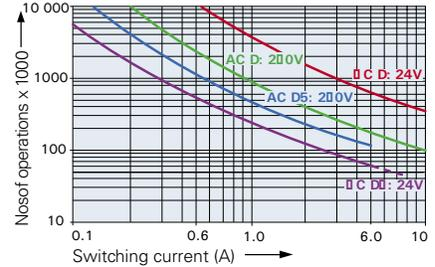
Max. switching characteristics (determined acc. to DIN EN 60947-5-1 table C2):
