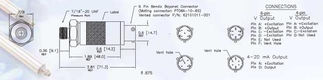
Vent through removed Pin F hole ( under 1000 psi ) Add 0.4" for CE EMI/RFI protection.
