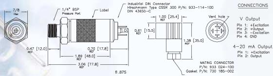
Vent through hole in connector ( under 1000 psi ) Add 0.4" for CE EMI/RFI protection.
