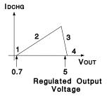
Region 1. When Vout = 0, the off time is infinite. This feature provides inherent short circuit protection. However, to ensure output voltage startup when the output is not a short, a high value resistor, Rs, is placed in parallel with Ct to establish a minimum switching frequency.
