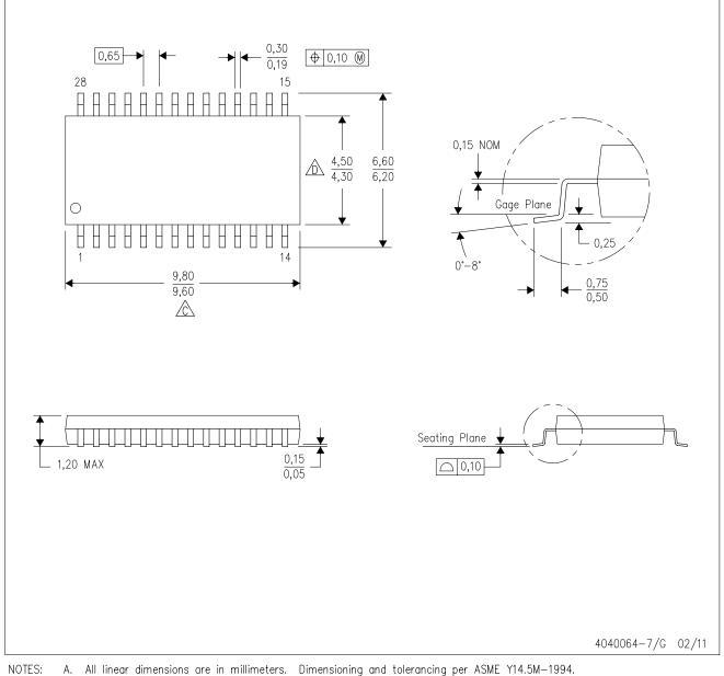
Ŗ. This drawing is subject to change without notice.  $\triangle$ Body length does not include mold flash, protrusions, or gate burrs. Mold flash, protrusions, or gate burrs shall
