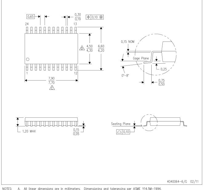
Α. All linear dimensions are in millimeters. Dimensioning and tolerancing per ASME Y14.5M-1994. Ŗ. This drawing is subject to change without notice.
