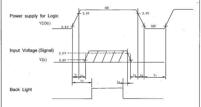
$\begin{array}{c} \underline{\text{POWER ON}} \\ & t_1 \leqq 15\,\text{ms} \\ \\ 0\,\text{ms} < t_2 \leqq 45\,\text{ms} \\ \\ 0. \ 1s \leqq t_3 \end{array}$
