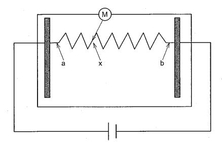
Va : maximum voltage in the active area of touch panel Vb : minimum voltage in the active area of touch panel
