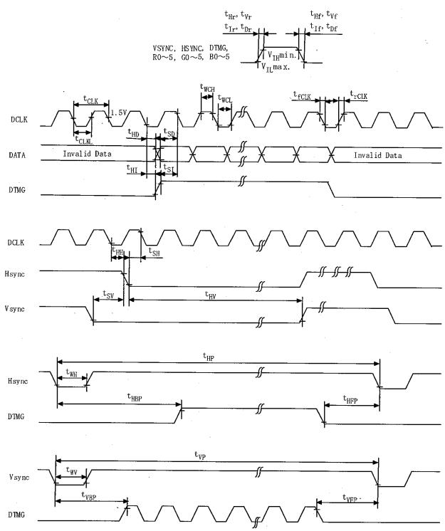
\*The DTMG signal for this module is defined as above-mentioned timings for Vsync and Hsync.
