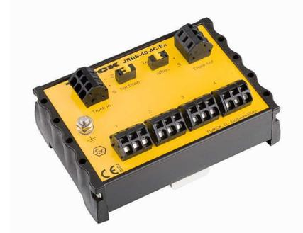
The 4-channel Ex junction box JRBS-40-4C/EX is designed for fieldbus systems according to IEC 61158-2, i.e. it is suited for both PROFIBUS PA and FOUNDATION™ fieldbus.
