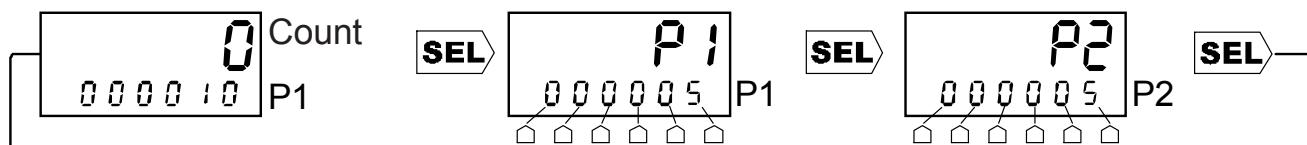
Press SEL, then use the Digit buttons to change P1. The display will flash. Press SEL again to accept the new P1 value, then use the Digit buttons to change P2. Press SEL again to accept the new P2 value. *If SEL is not pressed within 30 seconds of the last change to either P1 and P2, they will revert to their original values.*
