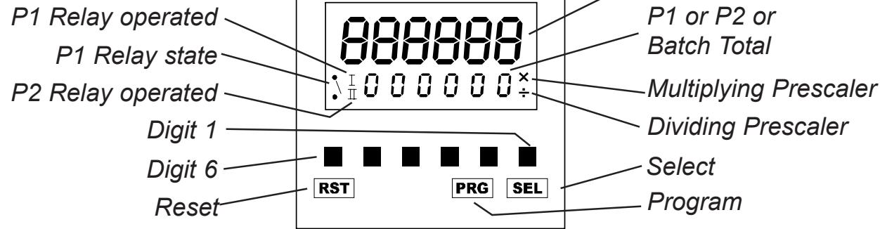
The front panel buttons are used to program the counter and to display and set the P1 and P2 presets. All the buttons can be disabled by the Keyboard Inhibit input. (see Programming, page 6).
