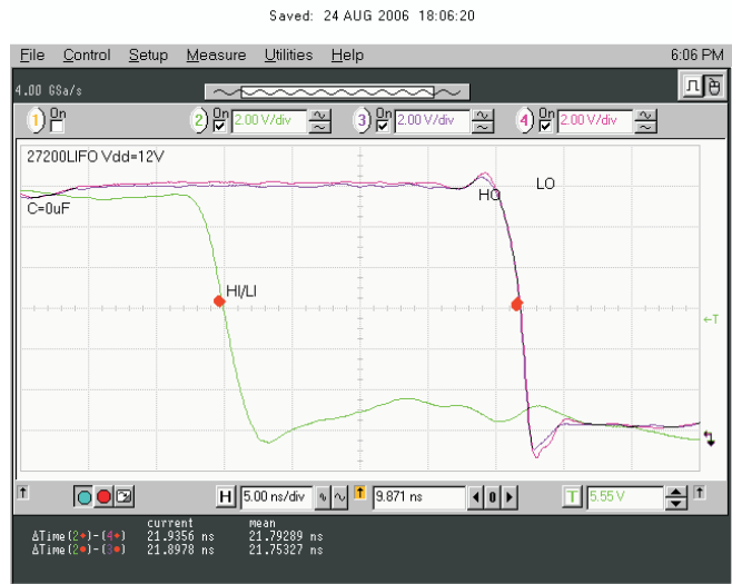
Figure 32. V_{LO} and V_{HO} Falling Edge Delay Matching
