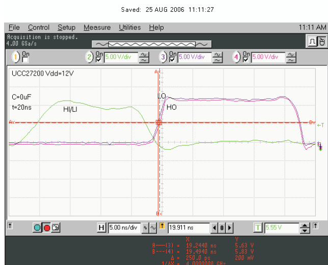
Figure 33. 20-ns Input Pulse Delay Matching
