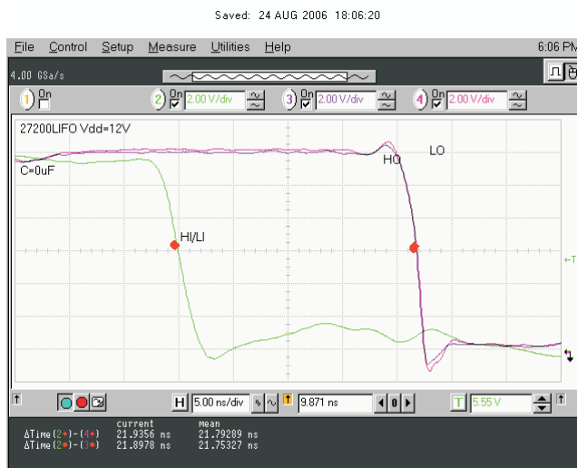
Figure 32. V_{LO} and V_{HO} Falling Edge Delay Matching
