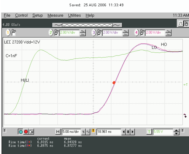
Figure 26. V_{LO} and V_{HO} Rise Time, 1-nF Load, 5 ns/Div
