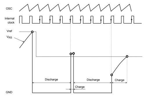
Transition from discharge mode to charge mode
