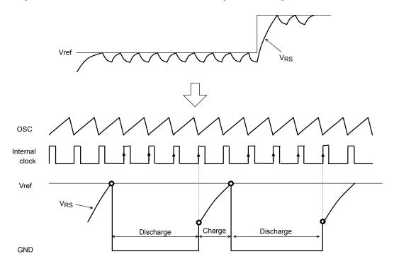
Transition from charge mode to discharge mode
