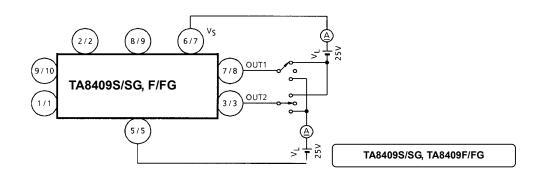
Test Circuit 5 V<sub>F U-1, 2</sub>, V<sub>F L-1, 2</sub>
