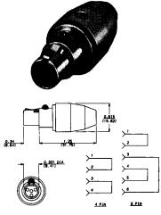
Looping plug is designed for circuit testing. Other inserts and wiring patterns are possible; contact Switchcraft.
