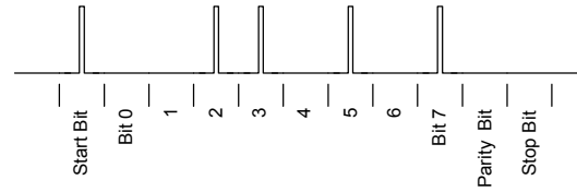
FIGURE 18-3 IrDA ASCII "S" with Odd Parity
