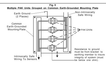
**Note:** All intrinsically safe wiring must be segregated from non-intrinsically safe wiring and shall have a minimum insulation thickness of .010".
