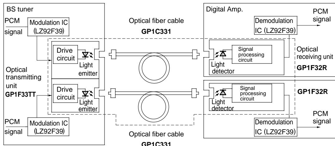
\*LZ92F39 is Sharp's modulation/demodulation IC.
