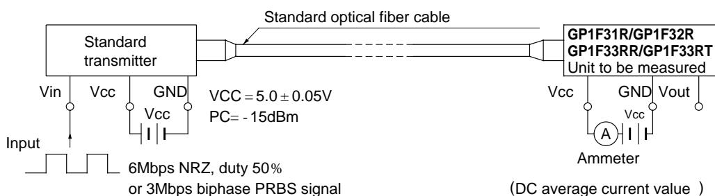
\*13 Output voltage/Pulse response measuring method
