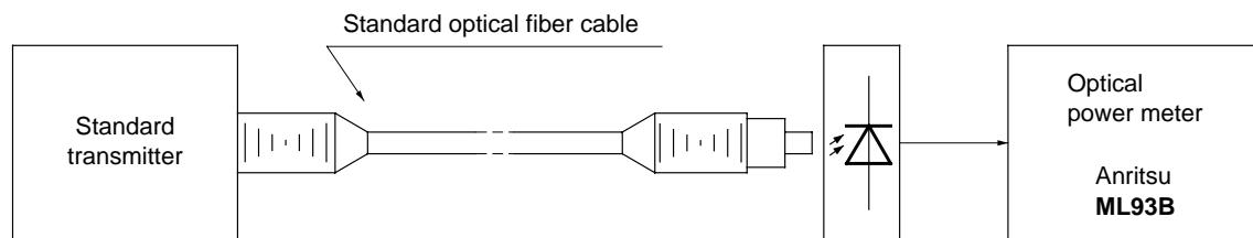
Standard light transmitter: Light transmitter that provides the fiber-end optical output of -15dBm ±0.3dBm when the standard optical fiber cable is connected.
