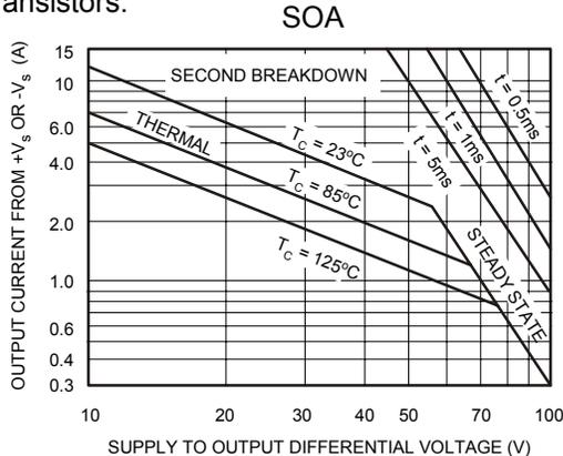
The SOA curves combine the effect of all limits for this Power Op Amp. For a given application, the direction and magnitude of the output current should be calculated or measured and checked against the SOA curves. This is simple for resistive loads but more complex for reactive and EMF generating loads. The following guidelines may save extensive analytical efforts.
