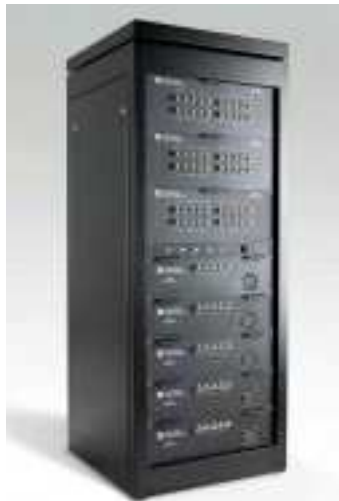
Base station cell site simulator equip.
