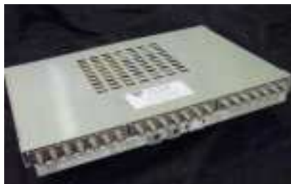
Receiver multicoupler and combiner
