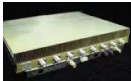
Base station simulator switch rack
