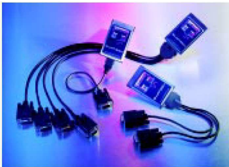
Quatech serial PCMCIA cards add one or two RS-232 or RS-422/485 ports to portable computers.
