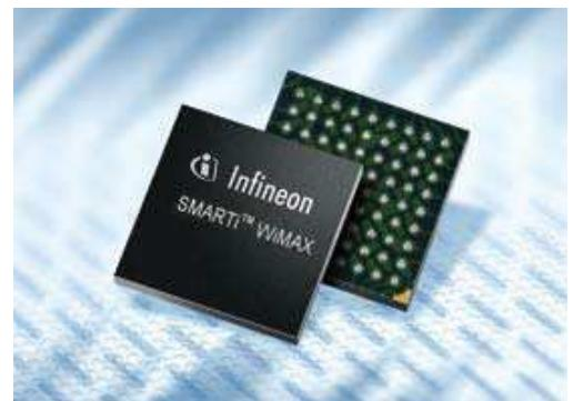
**SMARTi™ WiMAX (PMB 2008)** is the first single-chip dual-band WiMAX and WLAN Transceiver IC with standard I&Q interface for multi-media and feature-rich mobile devices.
