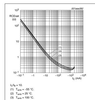
Fig.11 Equivalent on-resistance as a function of collector current; typical values.
