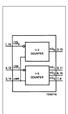
Fig.4 Functional diagram.
