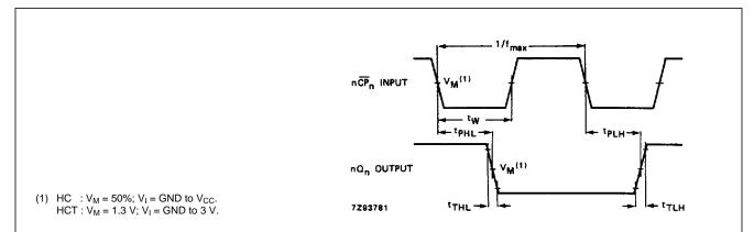
Fig.6 Waveforms showing the clock  $(n\overline{CP}_n)$  to output  $(nQ_n)$  propagation delays, the clock pulse width, the output transition times and the maximum clock frequency.
