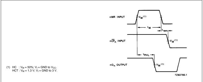
Fig.7 Waveforms showing the master reset (nMR) pulse width, the master reset to output (nQ<sub>n</sub>) propagation delays and the master reset to clock ( $\overline{\text{CP}}_n$ ) removal time.
