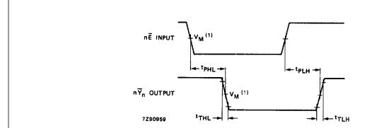
(1) HC :  $V_M$  = 50%;  $V_I$  = GND to  $V_{CC}$ . HCT:  $V_M$  = 1.3 V;  $V_I$  = GND to 3 V.
