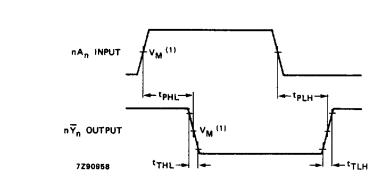
(1) HC :  $V_M$  = 50%;  $V_I$  = GND to  $V_{CC}$ . HCT:  $V_M$  = 1.3 V;  $V_I$  = GND to 3 V.
