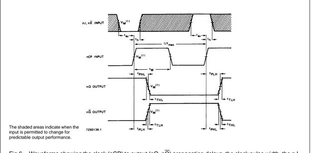
Waveforms showing the clock (nCP) to output (nQ, n $\overline{Q}$ ) propagation delays, the clock pulse width, the nJ, Fig.6  $n\overline{K}$  to nCP set-up, the nCP to nJ,  $n\overline{K}$  hold times, the output transition times and the maximum clock pulse frequency.
