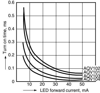
9.-2 Turn on time vs. LED forward current characteristics (AC/DC type)
