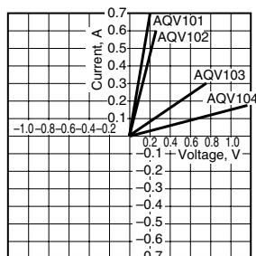
7.-2 Current vs. voltage characteristics of output at MOS portion (AC/DC type)
