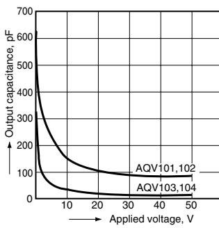
11.-2 Output capacitance vs. applied voltage characteristics (AC/DC type)
