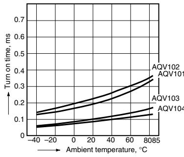
3.- (2) Turn on time vs. ambient temperature characteristics (AC/DC type)
