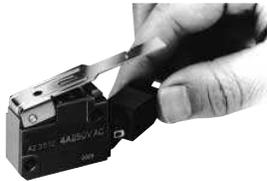
3) Connect lead wire to the receptacle terminals (#110) with insulating sleeve provided and insert it into the terminal of limit switch. (The lead wire can directly be soldered to the terminals without using receptacle terminals)
