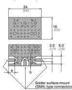
PC board for correction Dimensions (mm inch)
