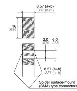
Material: Glass PTFE double-sided through hole PC board R-4737 (Panasonic Electric Works) Board thickness: t = 0.8 mm .031 inch Copper plating: 18  $\mu$ m Connector (SMA type receptacle) Product name: 01K1808-00 (Waka Manufacturing Co., Ltd.) Value has compensation PC board subtracted only for insertion loss. (Eliminate loss of connector and PC board.)
