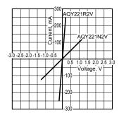
10. Off state leakage current vs. load voltage characteristics Measured portion: between terminals 3 and 4
