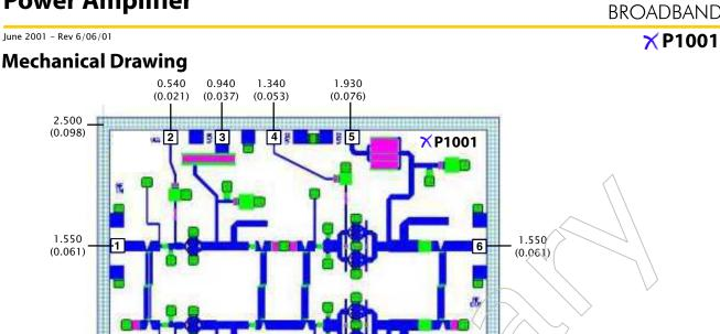
Units: millimeters (inches) Bond pad dimensions are shown to center of bond pad. Thickness: 0.100 (0.004) (for reference only), Backside is ground, Bond Pad/Backside Metallization: Gold All Bond Pads are 0.100 x 0.100 (0.004 x 0.004).
