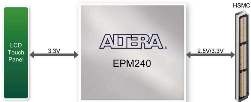
Figure 3-6 Block Diagram of the Bus Controller
