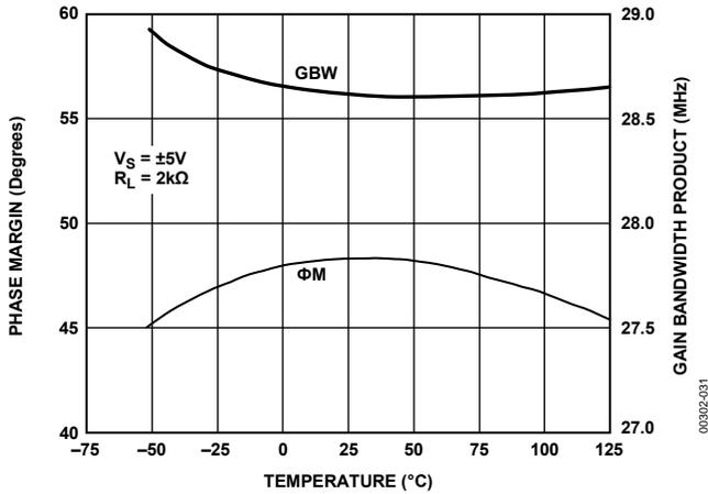
Figure 31. Phase Margin and Gain Bandwidth vs. Temperature
