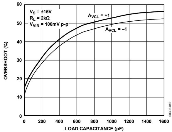
Figure 16. Small Signal Overshoot vs. Load Capacitance
