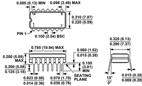
CONTROLLING DIMENSIONS ARE IN INCHES; MILLIMETER DIMENSIONS
