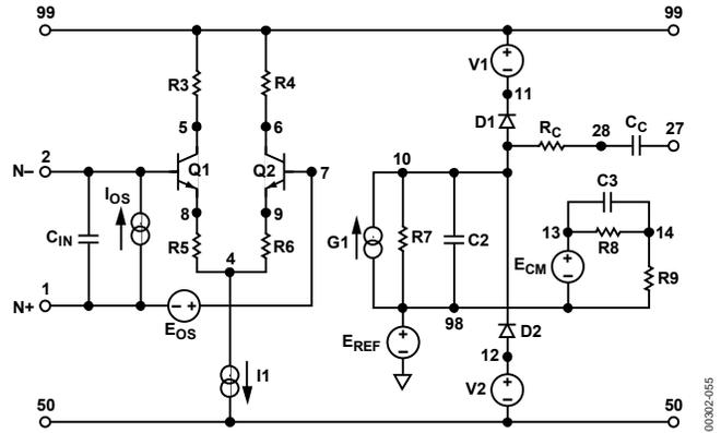
Figure 55. SPICE Macro-Model Input and Gain Stage
