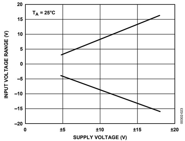
Figure 23. Input Voltage Range vs. Supply Voltage
