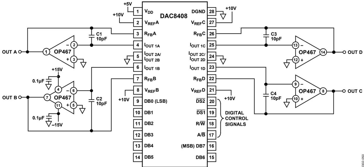
Figure 50. Quad DAC Unipolar Operation
