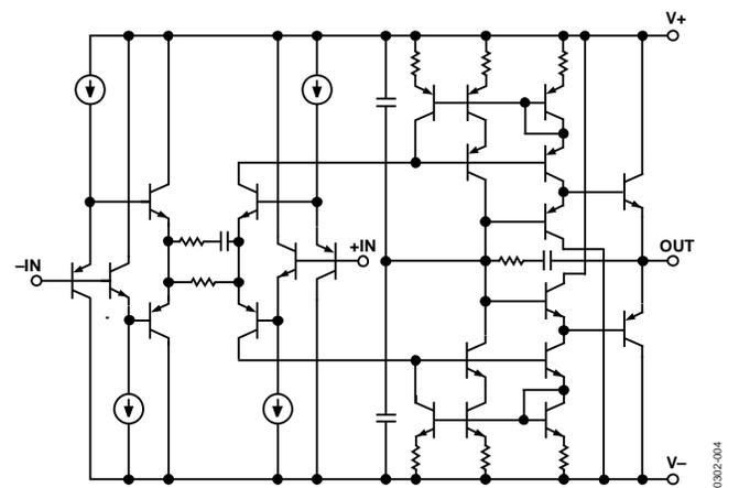
Figure 4. Simplified Schematic
