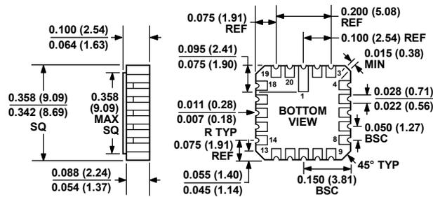
CONTROLLING DIMENSIONS ARE IN INCHES; MILLIMETER DIMENSIONS
