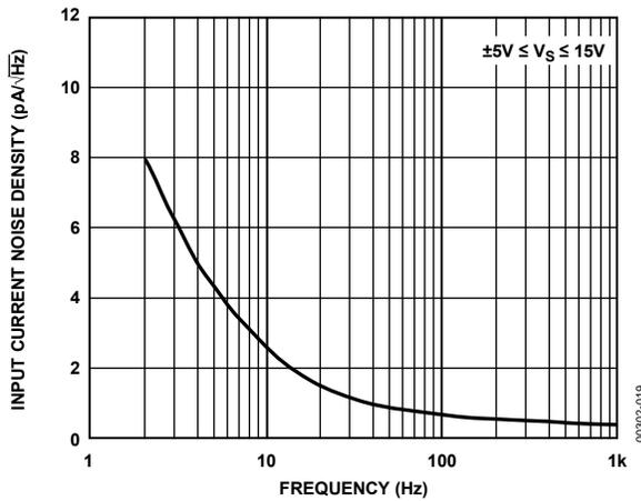
Figure 19. Input Current Noise Density vs. Frequency
