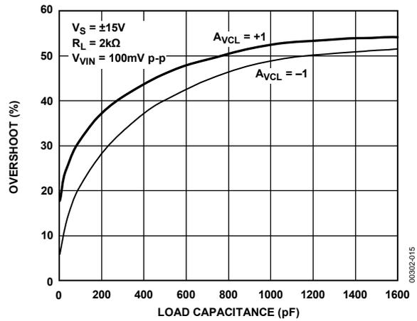
Figure 15. Small Signal Overshoot vs. Load Capacitance
