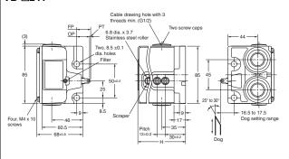
Note: Unless otherwise indicated, a tolerance of  $\pm 0.4$  mm applies to all dimensions.
