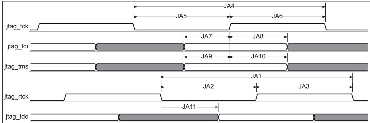
Figure 6-73. JTAG Interface Timing – Adaptive Clock Mode
