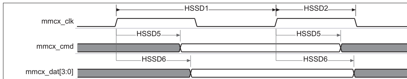
Figure 6-65. MMC/SD/SDIO – High-Speed SD Mode – Data/Command Receive
