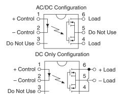
**Switching Characteristics** of Normally Open Devices
