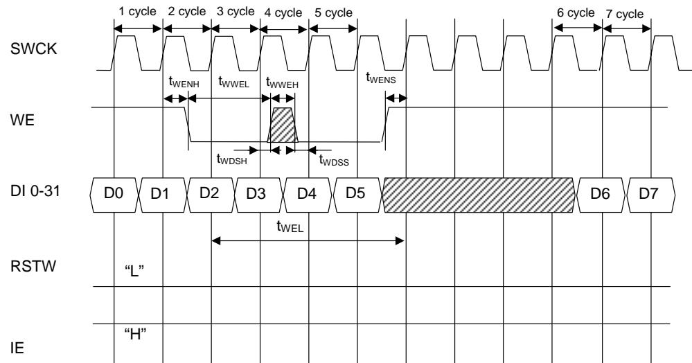
**Write Cycle Timing (Input Enable)**
