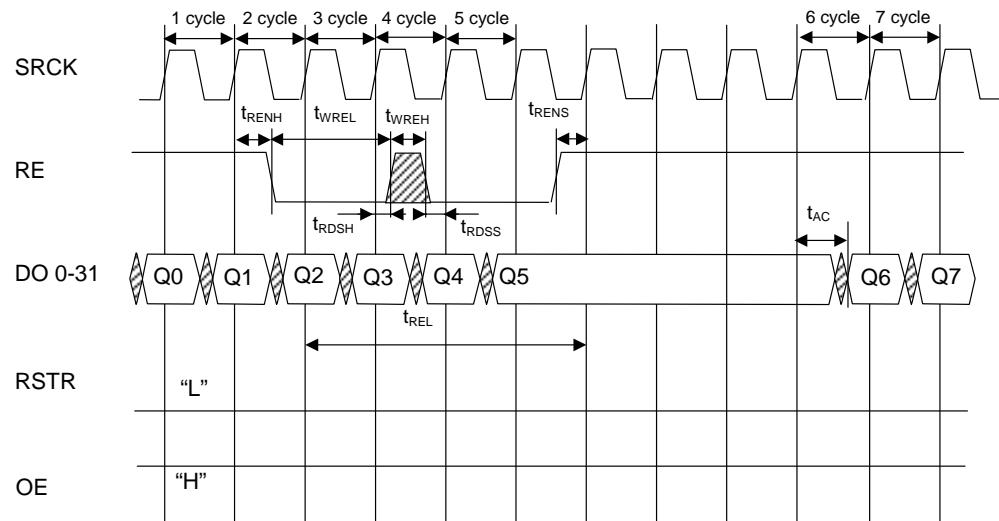
**Read Cycle Timing (Output Enable)**
