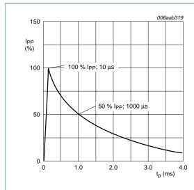
Fig 1. 10/1000  $\mu$ s pulse waveform according to IEC 61643-321
