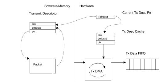
Figure 5-4 Transmit Architecture
