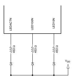
Figure 3-5 LED Loading Example
