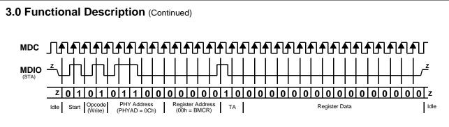
Figure 3-16 Typical MDC/MDIO Write Operation
