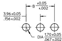
PCB LAYOUT: COMPONENT SIDE
