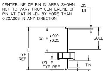
CENTERLINE OF PIN IN AREA SHOWN NOT TO VARY FROM CENTERLINE OF PIN AT DATUM -D- BY MORE THAN 0.20/.008 IN ANY DIRECTION.
