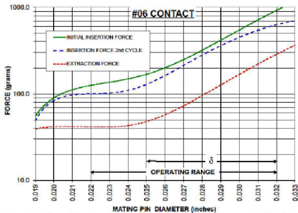
The insertion/extraction/normal force characteristics above were derived using 30 microinch gold plated contact and polished steel gauge pins having a bullet-shaped tip.
