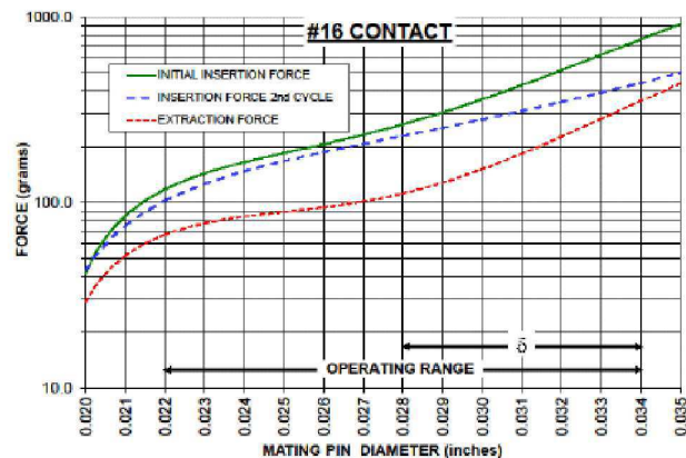
The insertion/extraction/normal force characteristics above were derived using 30 microinch gold plated contact and polished steel gauge pins having a bullet-shaped tip.
