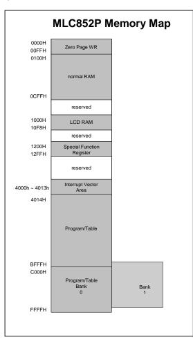
The address mapping of MLC852P is shown as below.
