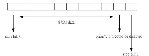
Each frame contains 10 or 11 bits depending on priority bit disabled or enabled
