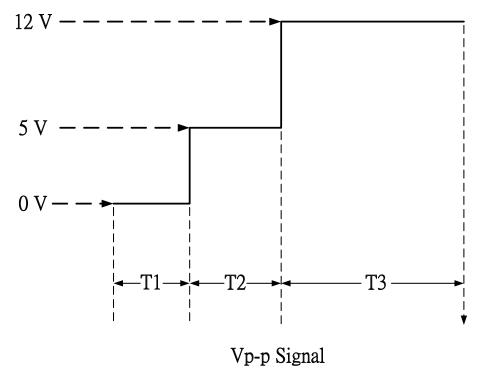
The voltage, waveform and timing requirments for VPP to program IC are as followed:
