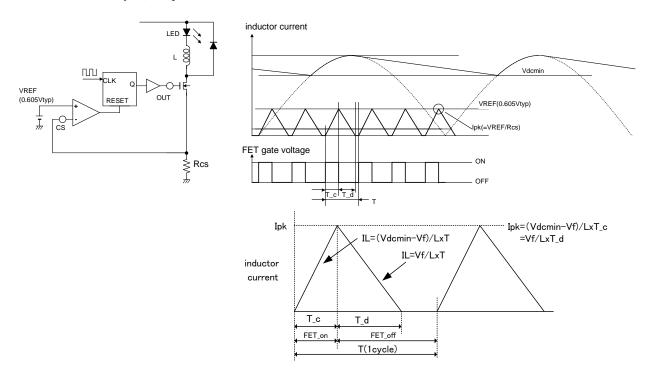
Given that the period when current flows into coil is  $DutyI = \frac{T_c + T_d}{T},$   $Ipk \times \frac{1}{2} \times (DutyI \times T)/T = ILED$   $Ipk = \frac{2 \times ILED}{DutyI} \quad (1) \text{ since } Ipk = \frac{VREF}{Rcs}$   $Rcs = \frac{VFET}{Ipk} = \frac{DutyI \times VREF}{2ILED} \quad (2)$
