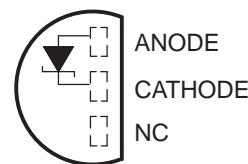
LP (TO-92/TO-226) PACKAGE (TOP VIEW)
