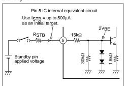
When an voltage of +5 V is applied to the mute pin through the external 15 k $\Omega$  resistor, the pin 6 voltage becomes about 1.85 V. (The muting function activation level in the specifications is 1.7 V minimum.) The pin 6 influx current (Imute) at this time will be roughly 210  $\mu$ A.
