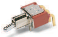
7101MD9ABE Horizontal Actuation SPDT
