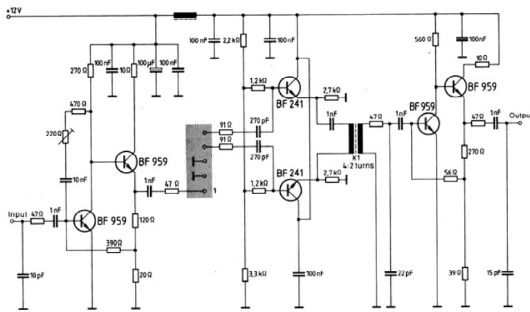
Test circuit for SIP-5 filter
