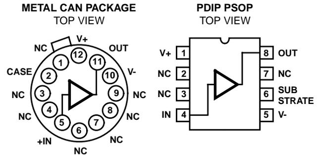
**FIGURE 1. HA-5033 PINOUTS: METAL CAN-PIN COMPATIBLE WITH THE LH0033 HYBRID. 8-LEAD, PDIP-FABRICATED USING A COPPER LEAD FRAME. ADVANTAGES INCLUDE EXCELLENT THERMAL CHARACTERISTICS AND BOARD SPACE SAVINGS.**
