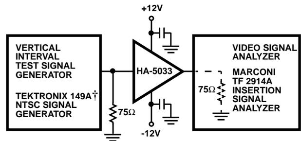
†TEKTRONIX 1910 NTSC DIGITAL GENERATOR RECOMMENDED
