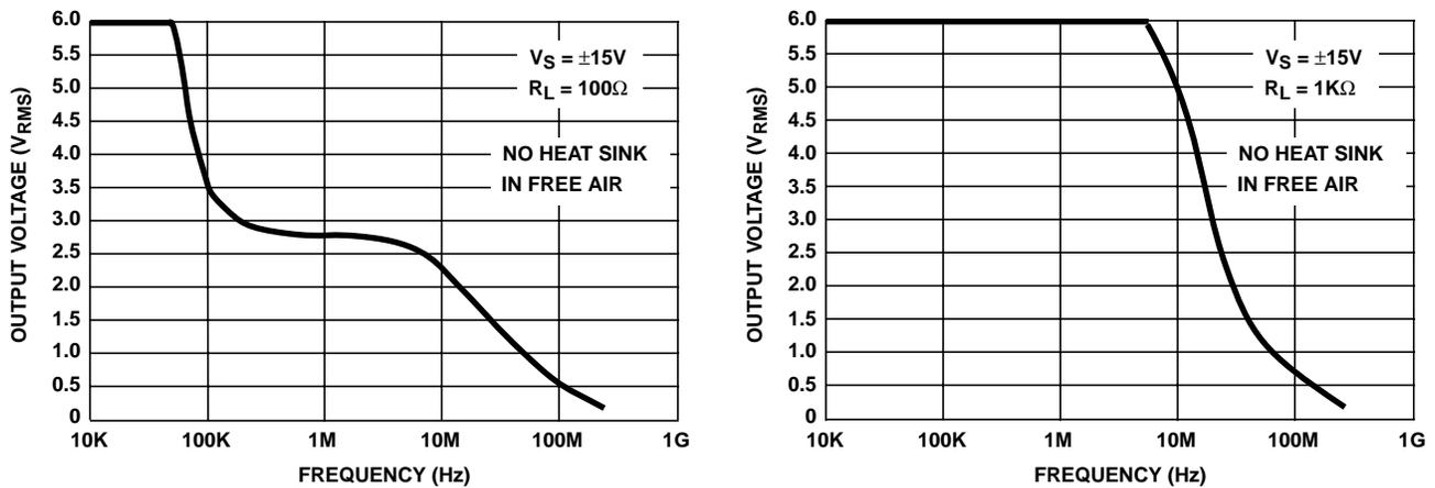
FIGURE 3. OUTPUT SWING vs FREQUENCY PERFORMANCE CURVES: CURVES SHOW POINT OF OBSERVABLE DISTORTION FOR GIVEN FREQUENCY. OPERATION BEYOND THE CURVES SHOWN WILL APPROACH CONDITIONS WHERE OUTPUT TRANSISTORS ARE SIMULTANEOUSLY ON. THE RESULTING INCREASE IN CHIP TEMPERATURE WILL LEAD TO THERMAL RUNAWAY.
