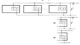
Note: H (Reset ON) level must be 4.5 V minimum.
