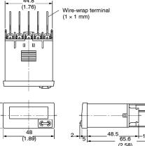
The wire-wrap terminals have a cross sectional dimension of 1x1 mm. Select one of three guages of wire from the table at right. Also listed in the table is the appropriate wiring hardware.
