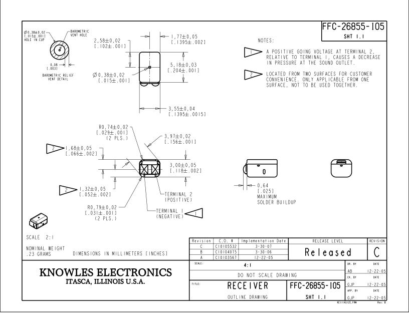
THE FFC-26855-105 IS A FERROFLUID, TYPE III DAMPED AND EXTERNALLY VENTED RECEIVER WITH A PEAK OF 5dB RELATIVE TO THE SENSITIVITY AT IKHZ UNDER CONSTANT VOLTAGE DRIVE CONDITIONS.
