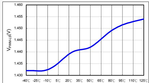
Figure 45. V<sub>PWM-LS</sub> vs. Temperature
