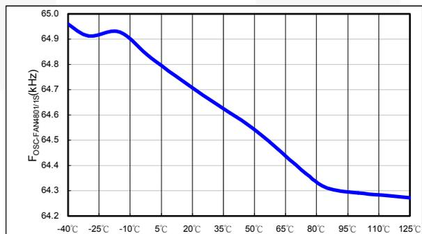
Figure 13. f<sub>OSC-FAN4801/1S</sub> vs. Temperature
