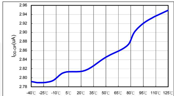
Figure 9. I<sub>DD-OP</sub> vs. Temperature
