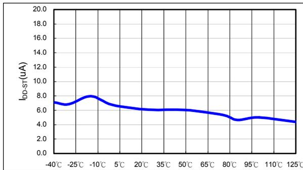
Figure 8. I<sub>DD-ST</sub> vs. Temperature
