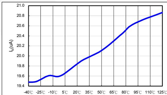
Figure 44. I<sub>IC</sub> vs. Temperature
