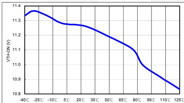
Figure 10. V<sub>TH-ON</sub> vs. Temperature
