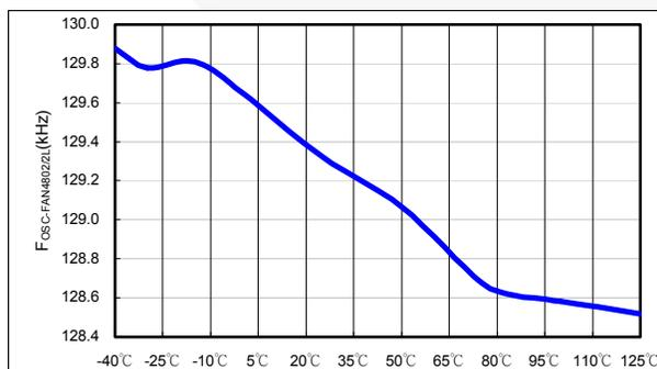
Figure 14. f<sub>OSC-FAN4802/2L</sub> vs. Temperature
