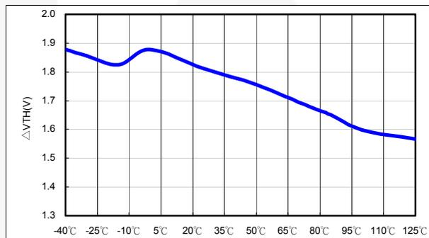
Figure 11. ΔV<sub>TH</sub> vs. Temperature
