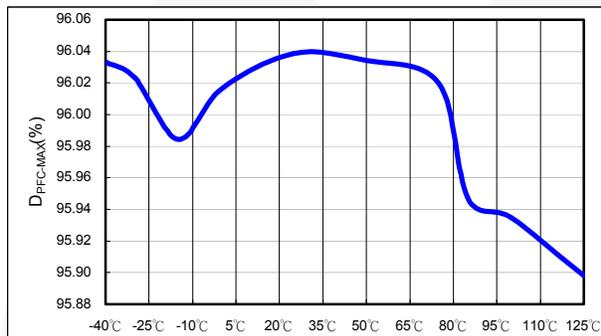
Figure 42. D<sub>PFC-MAX</sub> vs. Temperature
