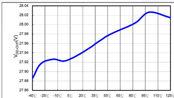
Figure 12. V<sub>DD-OVP</sub> vs. Temperature
