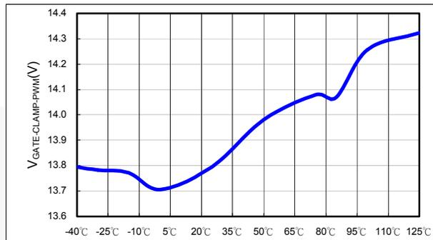
Figure 41. V<sub>GATE-CLAMP-PWM</sub> vs. Temperature
