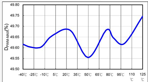
Figure 43. D<sub>PWM-MAX</sub> vs. Temperature
