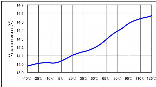
Figure 40. V<sub>GATE-CLAMP-PFC</sub> vs. Temperature
